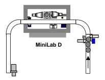
3.1.4 Off-Line – MiniLab D and MiniLab P – Single infeed conveyor
