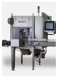
clamped at the neck, filled with water (optional capacity measurement is performed during the fill process), pressure tested, and then released to the cullet conveyor under the machine.
