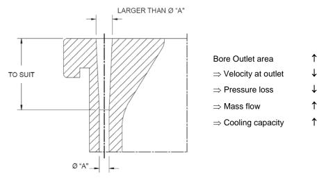
Figure 1 – Diffuser exit in mold
