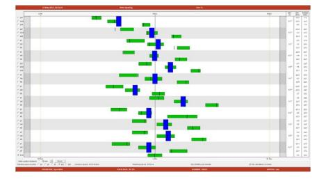
**Transport** – The transport provides information about how the actual ware spacing and ware positioning relates to the ideal positions on the conveyor belt.
