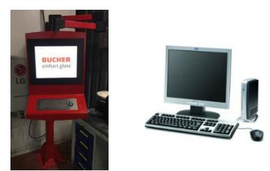
**Data server** -19" server computer that houses a database and a web server. The Data Server is connected to the customers LAN and installed in the server room in the glass plant. There is one data server for each plant that has a Blank or FlexRadar.
