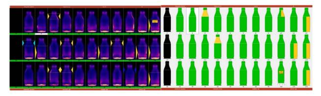
Last rejects and reject statistics – Using the reject information that the FlexRadar provides the user can identify problematic sections and cavities on the forming machine.
