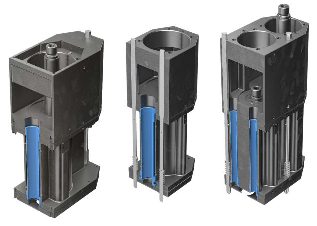
Plunger positioners are designed to suit the new plunger stroke. Optimized quick-change cartridges are also available, although the previous TG cartridge (62-3036) can be used as well.
