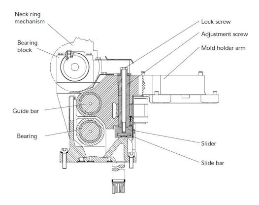
Blow Mold Support Mechanism
