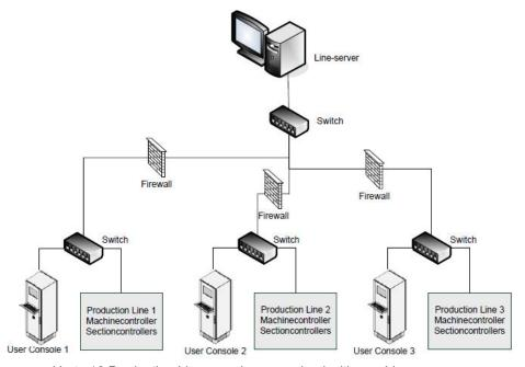
Up to 16 Production Lines can be supervised with one Line-server.
