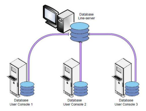
The Line-server is able to manage data up to 16 User Console Databases.
